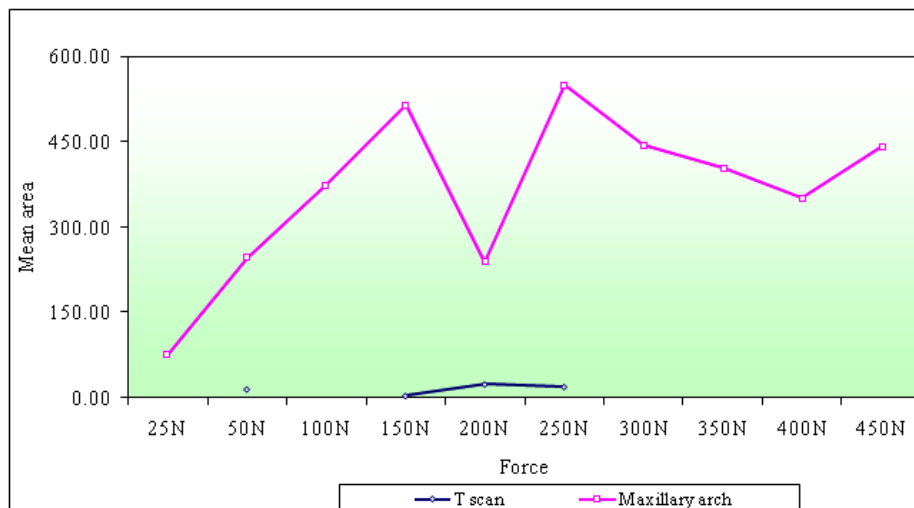
Figure 7. Comparison between results with articulating paper and T-Scan for applied load in the canine region.
