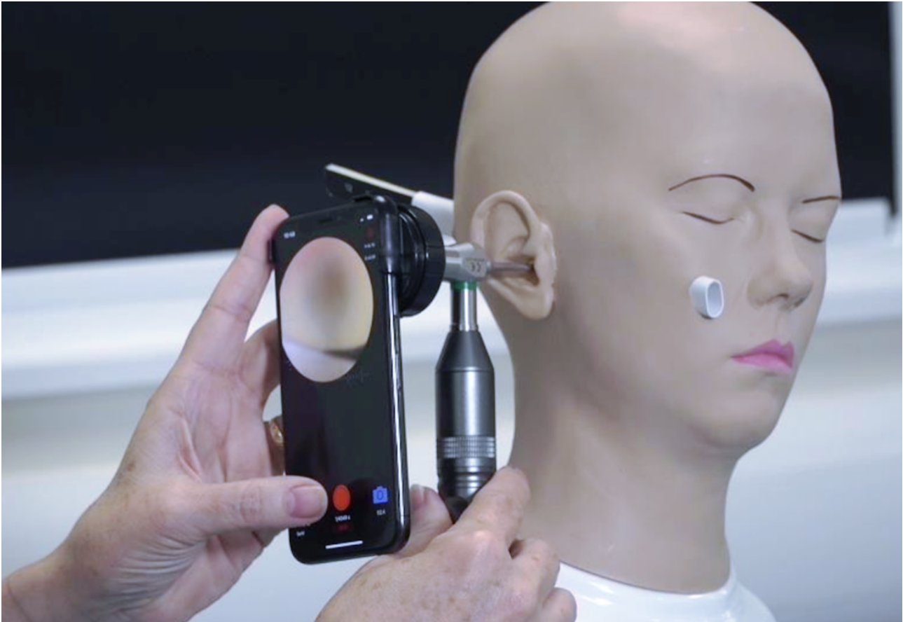
Figure 1. The endoscope-i in use on a mannequin head. Having a simple design, the product aims to be easy to assemble and use in various settings, including with outpatients, in general practitioner surgeries, and in the community.
