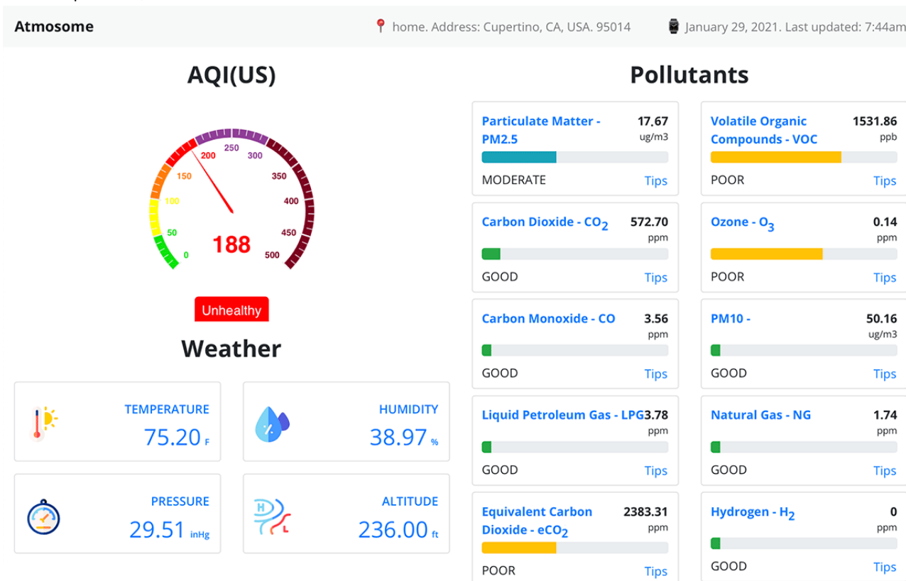
Figure 9. Representative example of hourly dashboard of user's atmosome data displayed by AMS UI. The values of 4 environmental parameters are also quantitatively presented below the AQI gauge. AMS: Atmosome Measurement System; AQI: Air Quality Index; PM 10 : particulate matter with diameter of 10 μm or less; UI: user interface.
