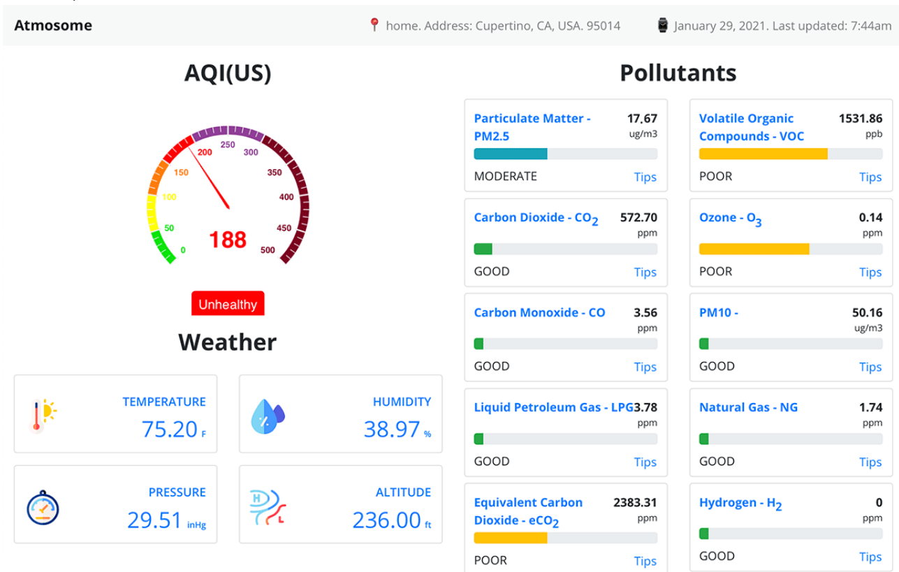
Figure 9. Representative example of hourly dashboard of user’s atmosome data displayed by AMS UI. The values of 4 environmental parameters are also quantitatively presented below the AQI gauge. AMS: Atmosome Measurement System; AQI: Air Quality Index; PM 10 : particulate matter with diameter of 10 µm or less; UI: user interface.
