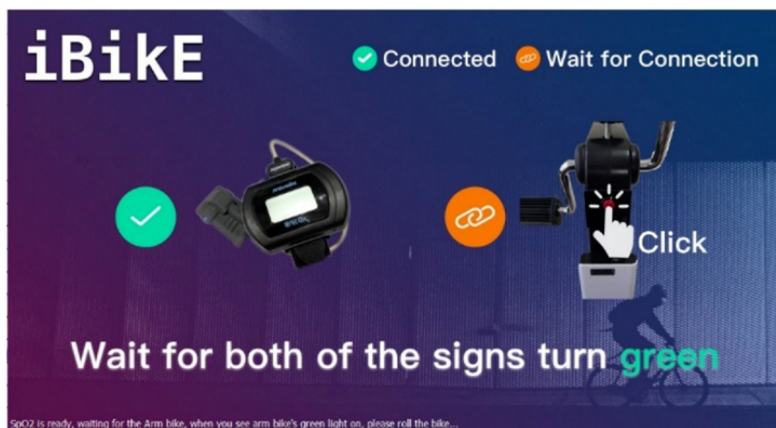
Figure 2. User interface. User needed to push a button to pair the application to the oximeter. They also needed to push the button on the right to pair the application to the iBike equipment to start the cycling session.
