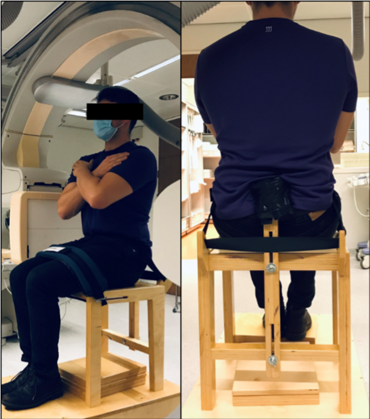
Figure 1. Customized wooden chair with 3-point fixation of the pelvis. The 3-point fixation is located on the anterior superior iliac spine, posterior inferior iliac spine, and the upper legs.
