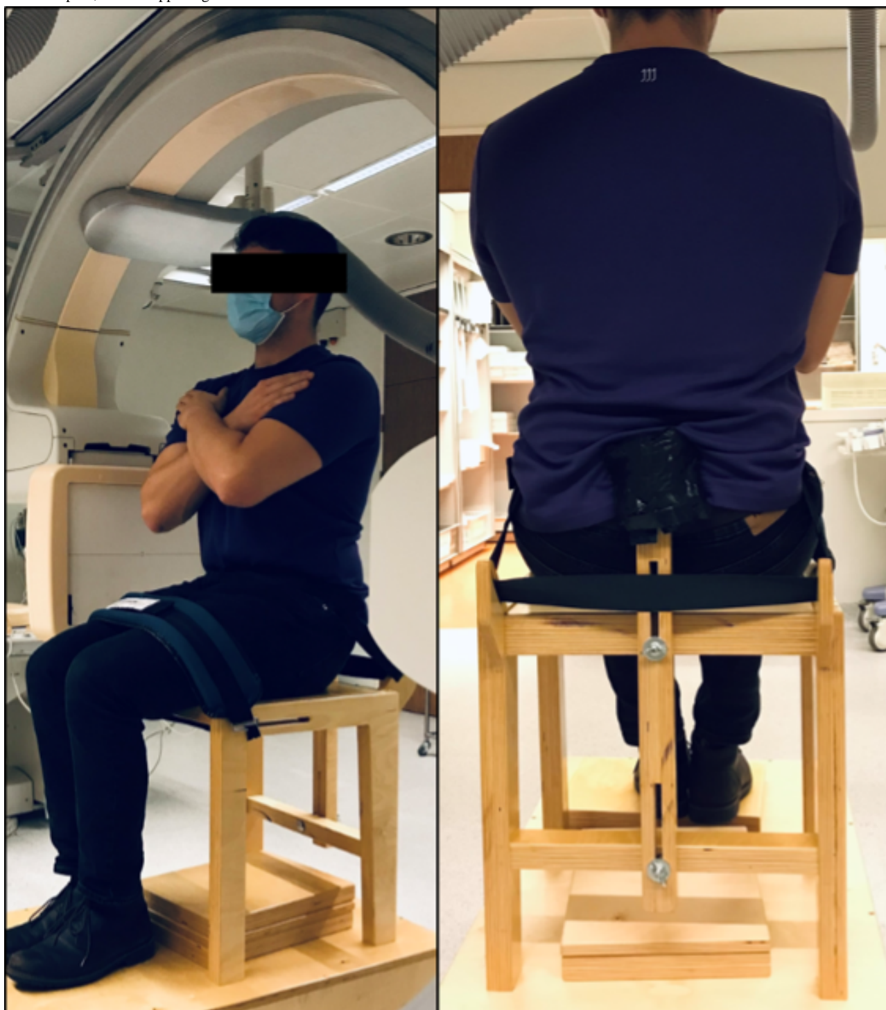
Figure 1. Customized wooden chair with 3-point fixation of the pelvis. The 3-point fixation is located on the anterior superior iliac spine, posterior inferior iliac spine, and the upper legs.
