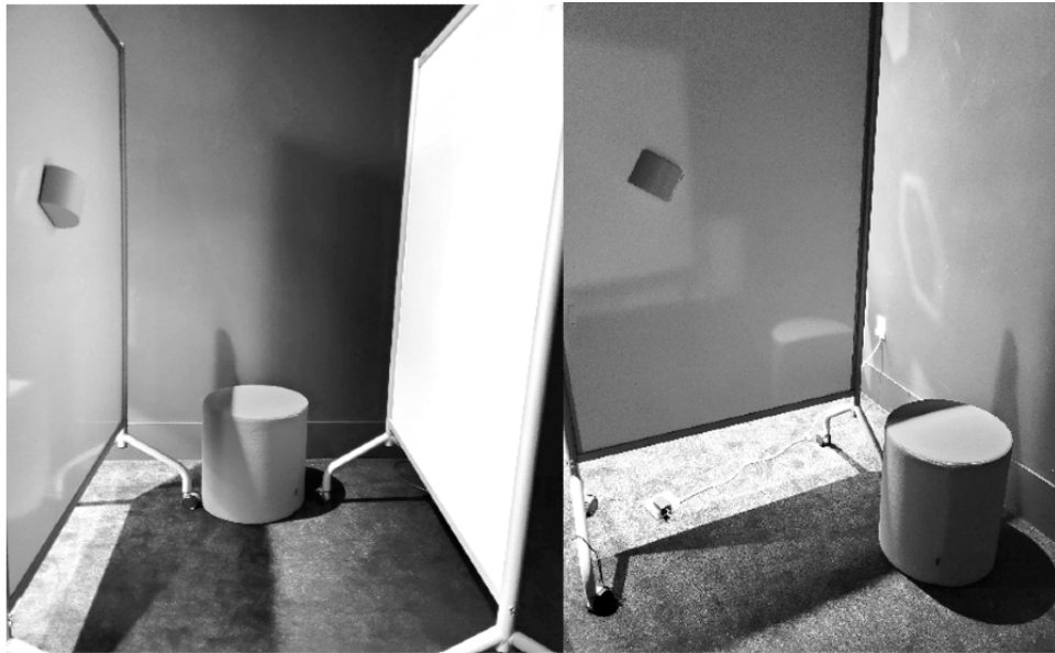
Figure 2. Mock restroom stall setup according to building code regulations (890-940 mm wide and 1500 mm long), with the toilet centered between the side walls.
