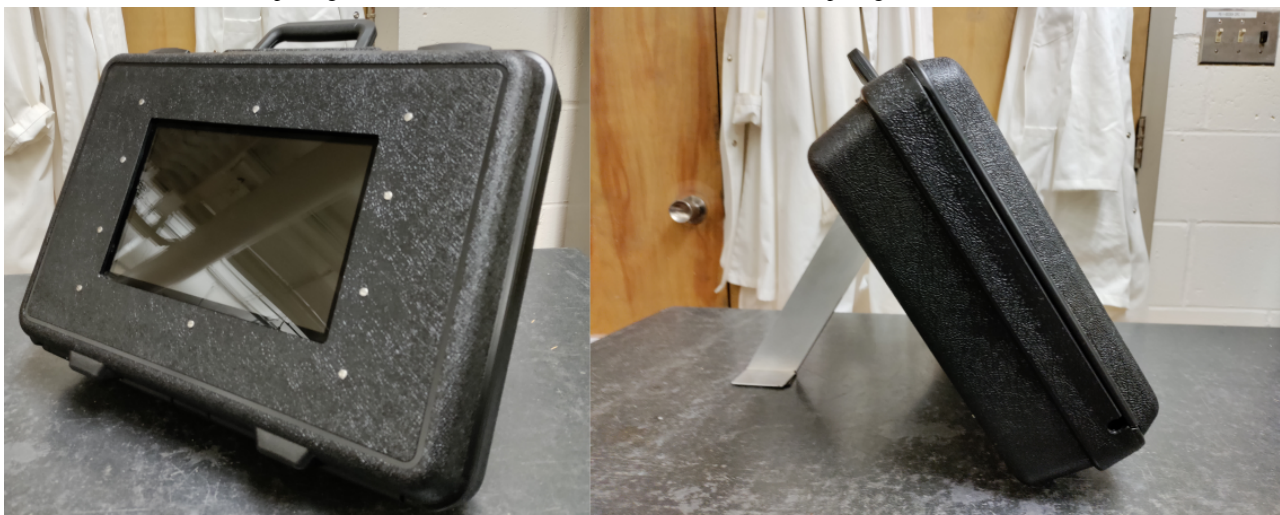
Figure 1. Pictures of the module packaged in a customized briefcase with a touch screen, computing unit, and hardware.
