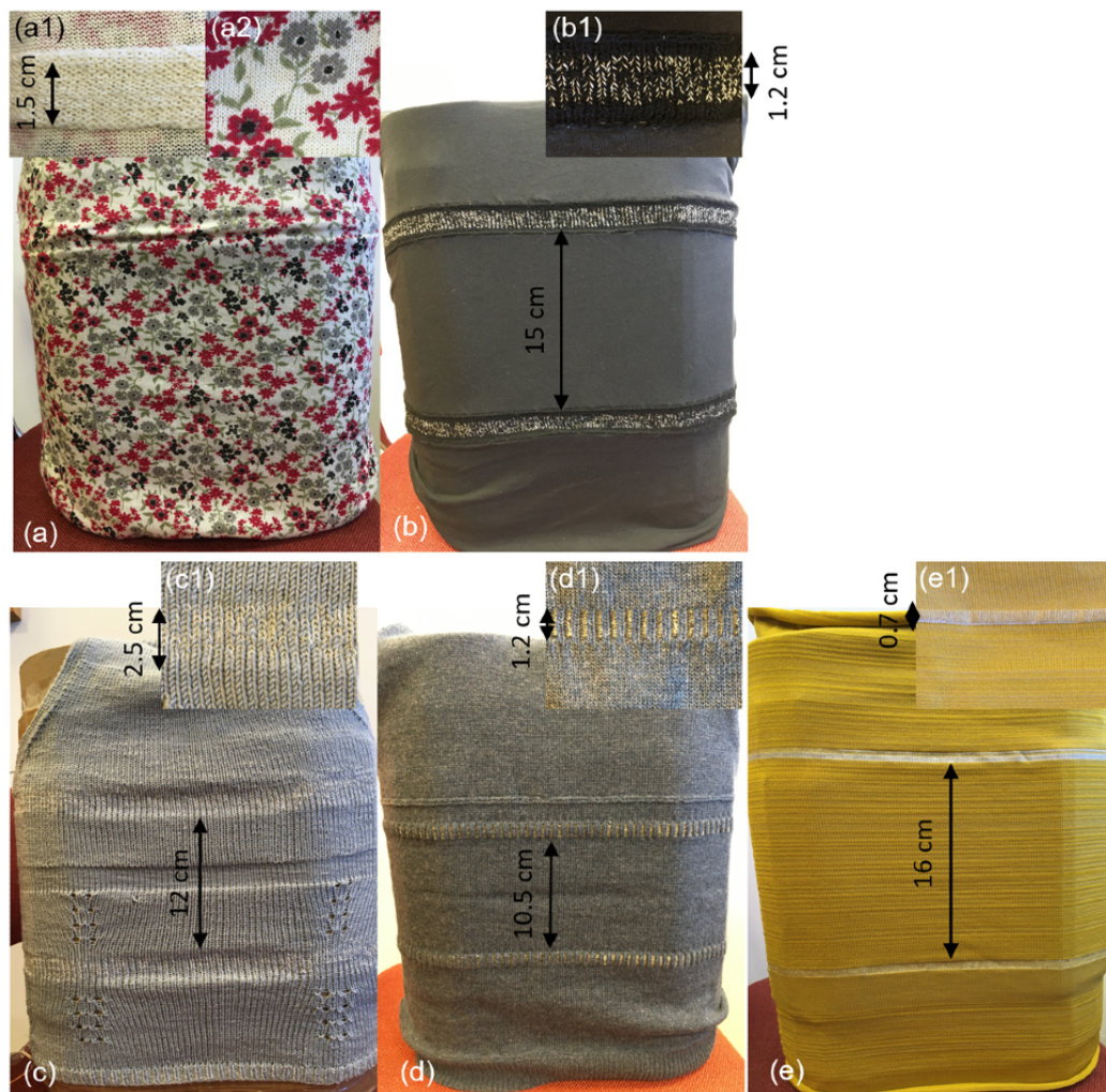
Figure 1. Pictures of the different implementations of the knitted sensor garment. The inset zooms in on the sensors. Top row: modular systems with knitted sensors are added to a garment. Bottom row: fully knitted implementations.
